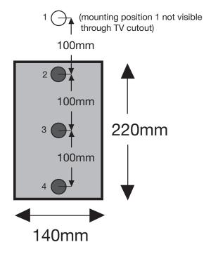
There are four mounting positions on the pole. The first hole cannot be used but the other three can. Position three is the default setting but if needed positions two and four can be used.
