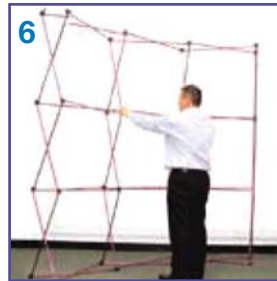
6 Add the mag bars onto the system for front, D-Ends and if applicable, the rear.
